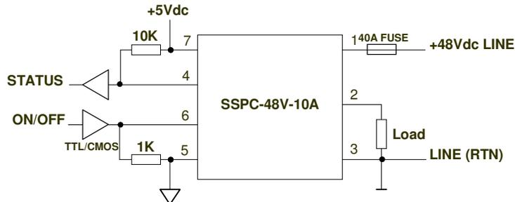
Figure 1.a – Normal OFF Control Connection
