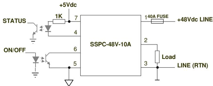
Figure 1.b – Normal ON Control Connection
