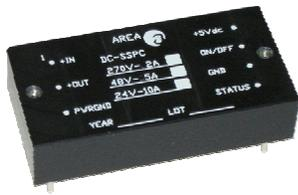
AREA Solid State Power Controller (SSPC) Modules combine the functions of a circuit breaker, including load monitor and I<sup>2</sup>t protection, in a small and cost effective plug-in package, without any internal mechanical part that can wear out.
